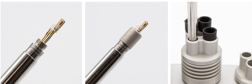
Figure 37 HMP5 calibration with HMK15 using 211302SP adapter
