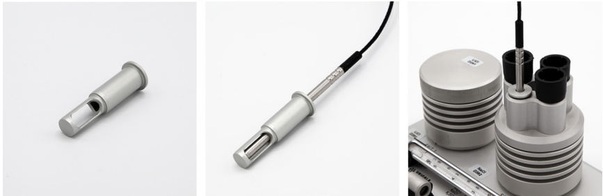
Figure 38 Using HMP9 calibration adapter with HMK15
