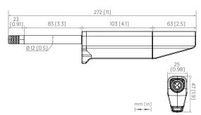
Dimensions of HMP80L (top) and HMP80N (bottom), side and bottom view
