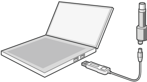
Figure 15 Connecting Probe to Insight
