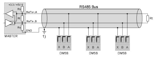
One ground connection only. This is possibly made within the master (PC). Rt: Termination resistors: 120  $\Omega$  each for long cables (> approx. 10 m)
