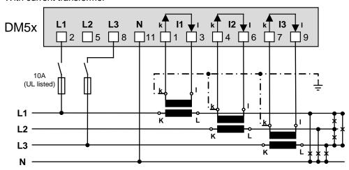
• With current and 2 single-pole isolated voltage transformers
