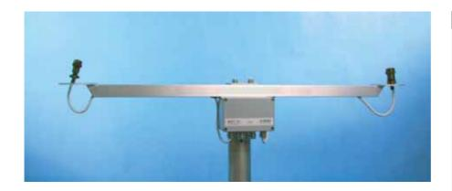
The Vaisala Wind Transmitter WAT12 is an economic solution to a standard interface between Vaisala's wind sensors and analog panel meters, chart recorders, digital LCD or LED displays, data loggers, computers with analog inputs, etc. The transmitter converts the wind speed and direction data measured by either Vaisala Wind Set WA15 or Vaisala Wind Set WA25 into two analog current loop signals, respectively. The power to the sensors is also supplied through the WAT12 unit.
