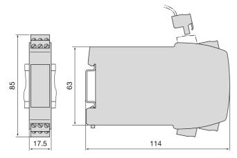
Fig. 12. SINEAX V624 in housing P12/17 St clipped onto a rail "G" (35 × 15 mm or  $35 \times 7.5$  mm, acc. to EN 50022), screw terminals pluggable.
