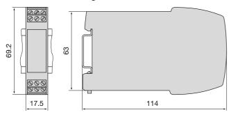
Fig. 11. SINEAX V624 in housing P12/17 clipped onto a top-hat rail (35  $\times$  15 mm or  $35 \times 7.5$  mm, acc. to EN 50022), screw terminals not pluggable.
