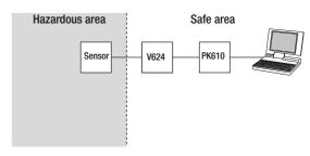
Fig. 7. Configuring the SINEAX V624, types 624-33/34/93/94, when the sensor is in the hazardous area. For this case the switch on the interface of the PK610 must be set to "ON" or "OFF", see Fig. 6.
