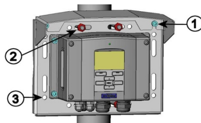
Figure 15 Mounting Rain Shield with Installation Kit
