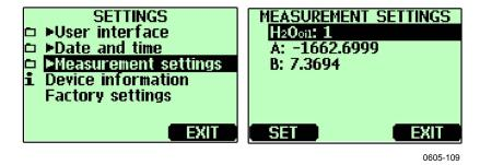
Figure 15 Measurement Setting Menus
