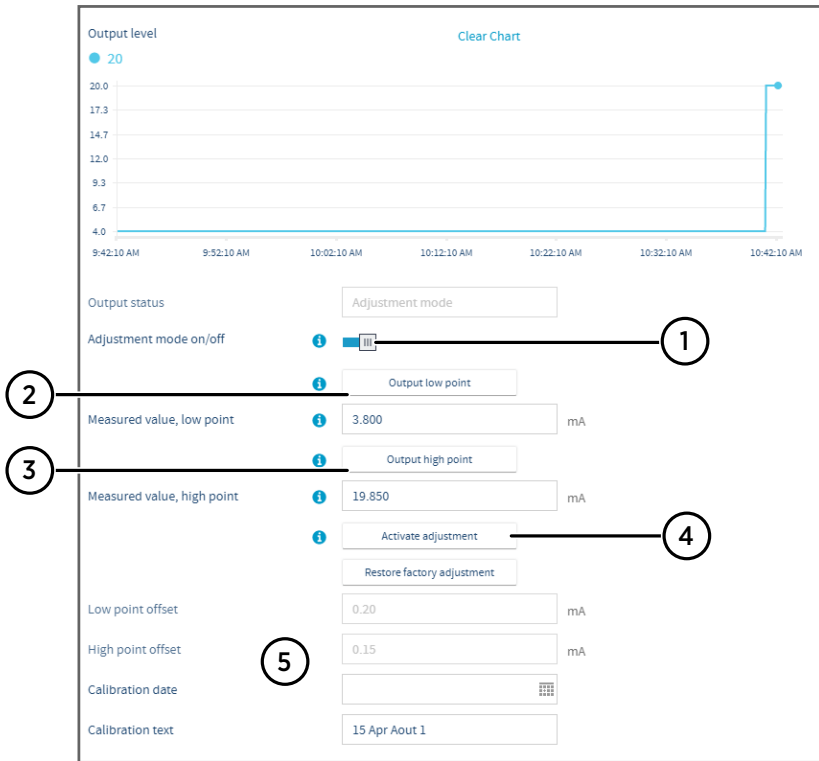
Figure 46 Analog output level adjustment in Insight PC software
