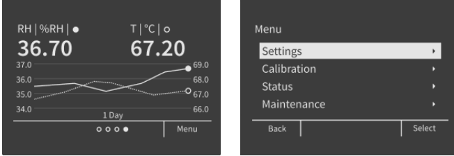
Figure 23 HMT370EX local display examples: measurement graph view and main menu screen
