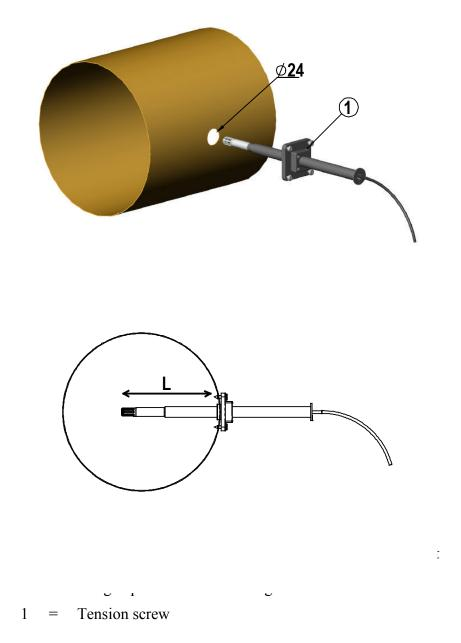
Distance L can be adjusted and locked in place with the tension screw.
