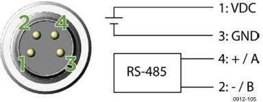
Figure 21 Wiring of Digital Output
