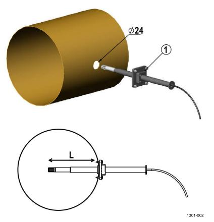
Figure 10 Probe Installation with the Duct Installation Kit
