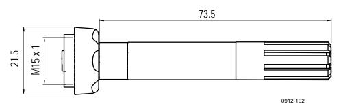
Figure 17 HMP63 and HMP113 with Plastic Locking Bushing, Dimensions
