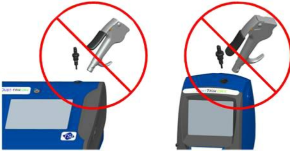
Figure 4-3: Do NOT Blow into Instrument
